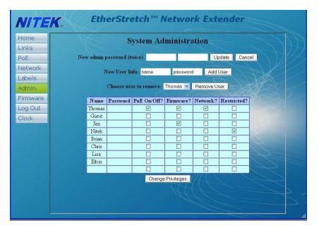
Also available only in the ADMIN screen is the CLOCK button. This can be used to set the current time internal to this unit only. Set the current time for the unit in this screen. There is a real time clock in the unit which is battery backed up. It is unlikely that the battery would need to be replaced under normal use but if it did the battery type is a standard CR1220. The battery must be replaced by a qualified service tech only.
