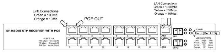
Front Panel Jacks and LEDs
